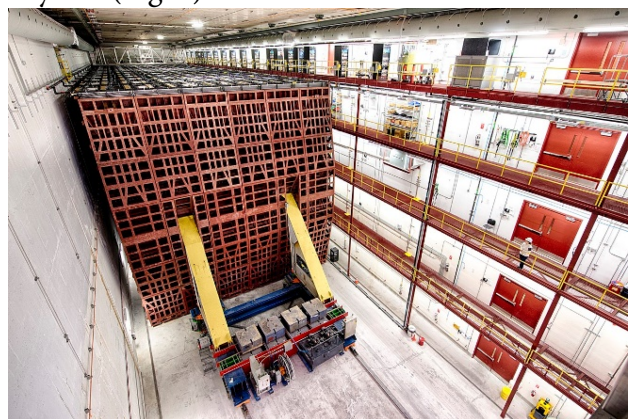
Figure 3: NOvA’s 4-storey neutrino detector. NOvA researchers fire a beam of neutrinos from Fermilab, IL, through 810 km of solid Earth, to this detector located in Ash River, MN. The long distance allows neutrinos to oscillate between flavor states. 6
