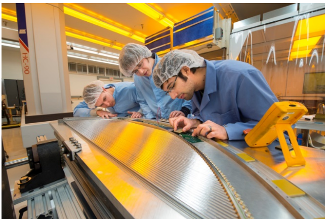
Figure 2: Researchers carefully construct a Mu2e detector module. Center is UMN post-doc Dan Ambrose. Undergraduates at UMN are helping to build 250 of these detectors. 4
