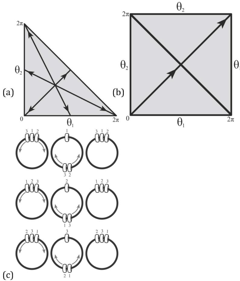
FIGURE 8. Periodic 2-bounce bead orbits and schematic collision diagrams. (a) The three different 2-bounce orbits in the triangle; (b) The 2-bounce orbit in the reflected triangle; (c) Schematic diagrams of the three bead 2-bounce orbits on the ring.
