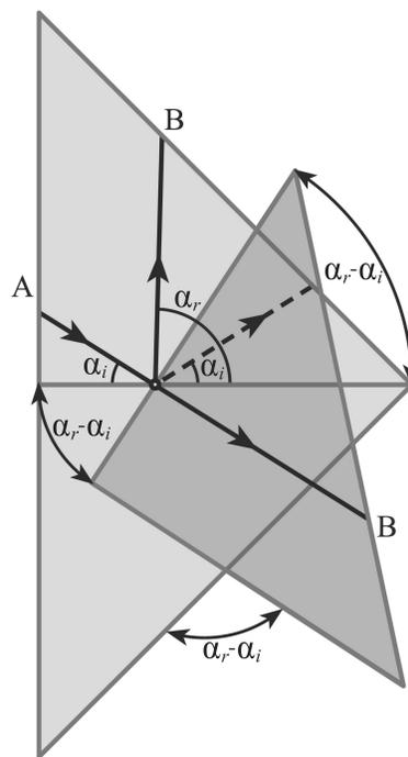
FIGURE 11. Method of reflection and rotation for the bead collisions. The orbit is drawn as a straight line with two segments. The second segment is drawn in a reflected and rotated triangle, where the reflected triangle is about the collision side, just like the billiard problem. However since the reflection is non-specular, the triangle must be rotated by angle  $\alpha_r - \alpha_i$  to compensate for the difference between the specular reflection and the non-specular reflection.
