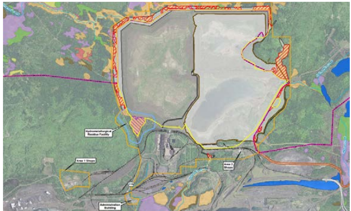
Figure 3. Map of directly impacted wetlands at plant site. This map depicts part of the 912.5 acres of wetland areas lost directly to the project, at the plant site. The area outlined in orange is the plant site, and red checkered areas represent wetlands directly lost. The various other shaded areas represent different wetland types surrounding the plant that include those indirectly affected. Figure from (MNDNR 2013).
